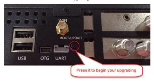
4. Unpack the firmware file then run "MfgTool2.exe", click "start" to burn the new firmware, after finished, power off MOI Pro, press down boot switch button, and then you can enjoy the new OS.
