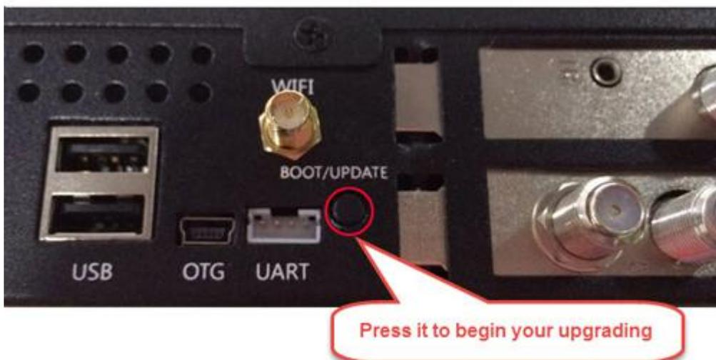
4. Unpack the firmware file then run "MfgTool2.exe" , click "start" to burn the new firmware, after finished, power off MOI Pro, press down boot switch button, and then you can enjoy the new OS.
